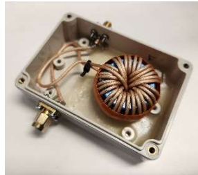
Home-made common-mode transformer
