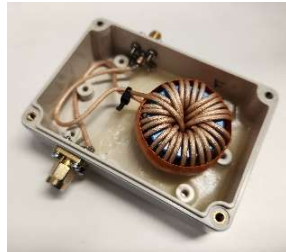
Home-made common-mode transformer
