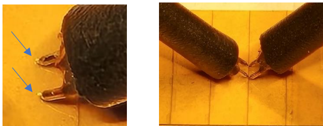
Figure 14: Planarizing (left) and aligning (right) the probe tips.
