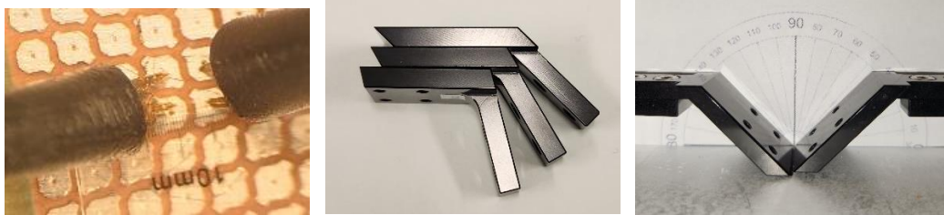
Figure 16: Illustration of probe spacing measurement with a thin plastic ruler using 0.1mm marks (left), choice of landing-angle adaptors (middle) and illustrating the checking of landing angle adaptor angle mounted on probe holders (right).
