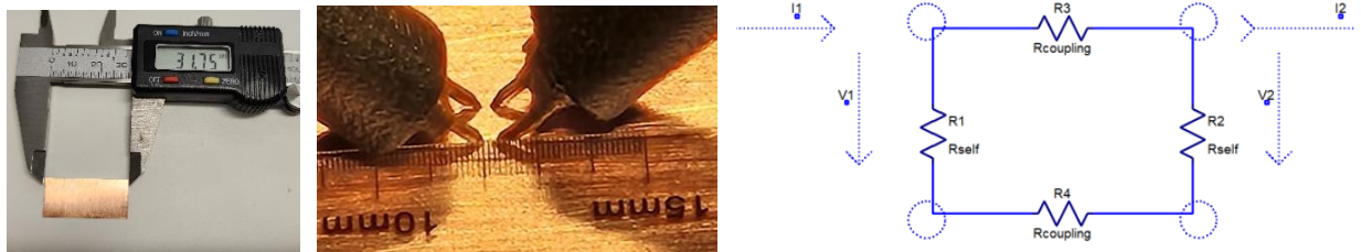
Figure 5: Photo of the copper sheet (on the left) and probes landed on the sheet with microscale (in the middle) and DC equivalent circuit (on the right).
