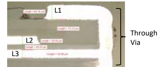
Test board stack up cross section.
