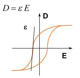
Class II and higher ceramic materials are ferroelectric Ferroelectric materials have saturating hysteretic D-E curves  $\epsilon$  and C are voltage dependent!
