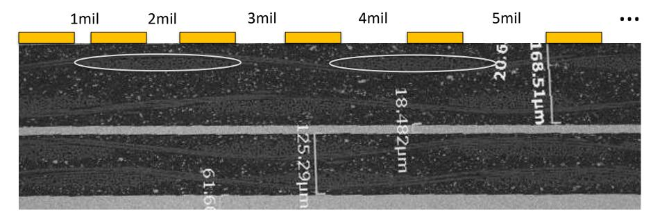
Offset to avoid tight trace coupling and accommodate probing footprint
