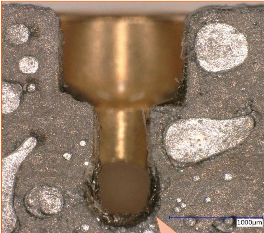
Sure enough, solder was found pooling along the inner edge of the connector at the pad
